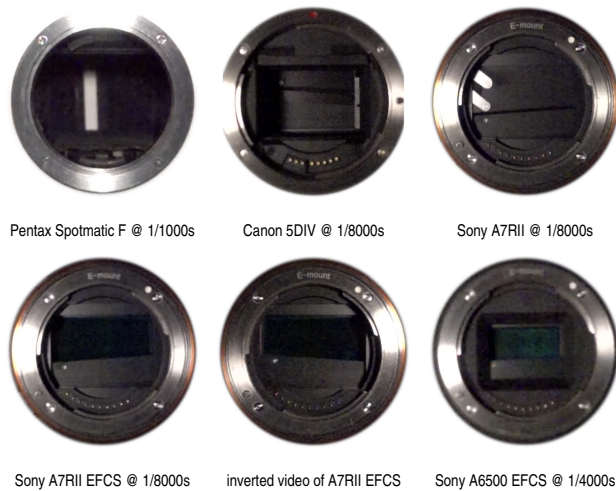
Figure 5. High speed images of focal plane shutters
