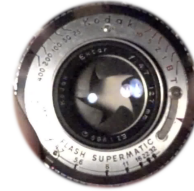
Figure 1. Still image from high speed video of leaf shutter
