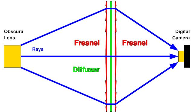
Figure 11. BSI DCO with Fresnel screen sandwich (not to scale)
