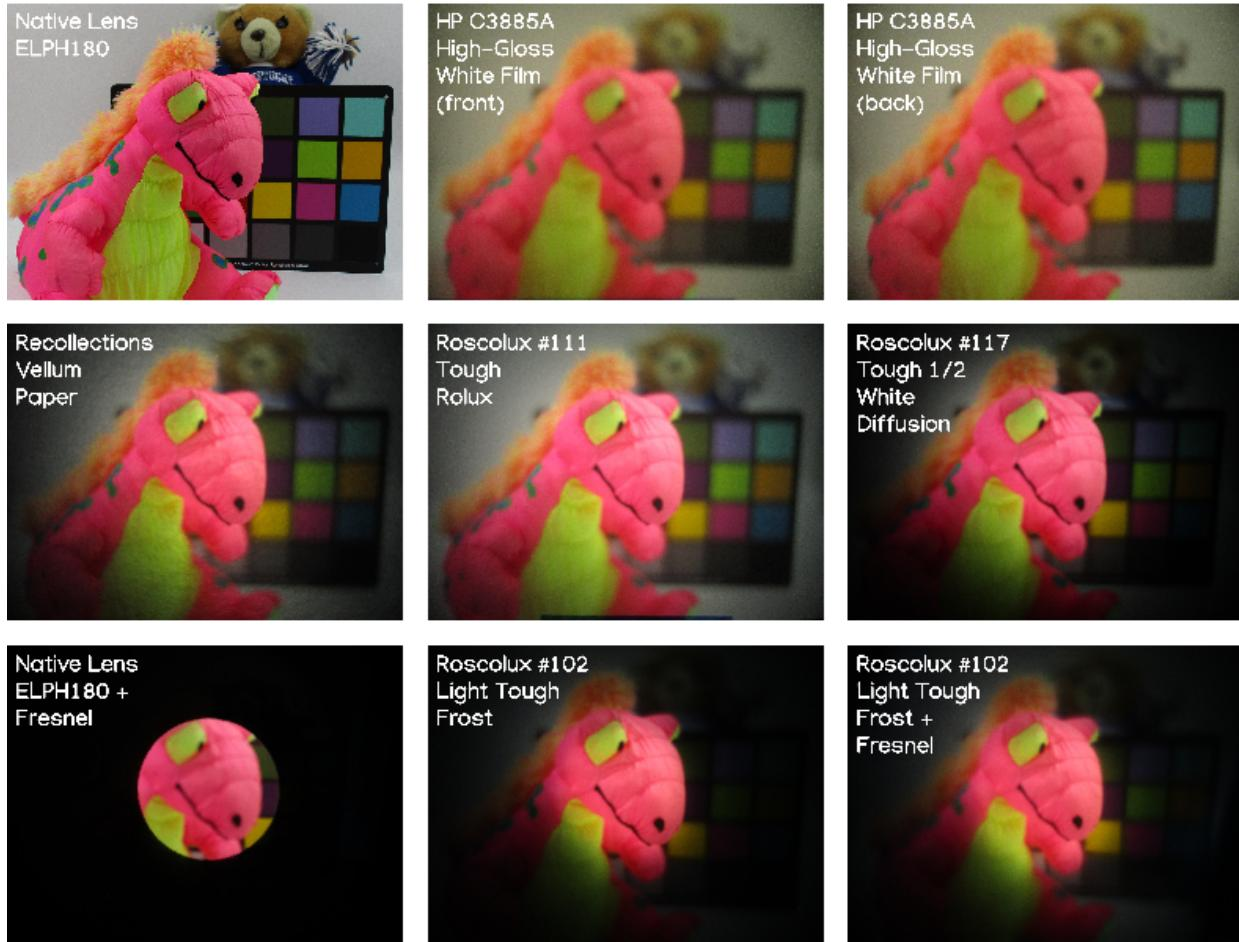
**Figure 12.** Test scene BSI DCO images using various screens with ELPH180 on CHEM with SMC Takumar 50mm f/1.4
