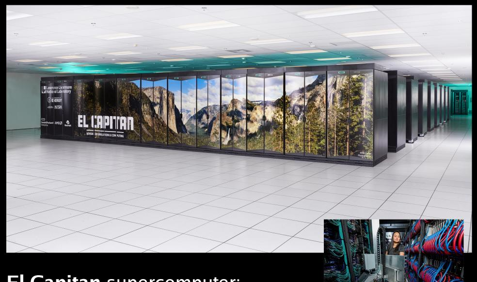
El Capitan supercomputer: 11,039,616 cores, 2.746 Exaflop/s Cost approx. \$600M, 29.6 MW power
