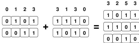
Fig. 2. Addition of two 2-pbit values
