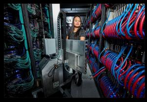
El Capitan supercomputer: 11,039,616 cores, 2.746 Exaflop/s Cost approx. \$600M, 29.6 MW power
