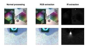
**Multispectral Imaging.** In the process of trying to remove chromatic abberations, we found a way to extract multispectral data from a single raw capture using an unmodified digital camera (a CANON G1 for the above). We have continued to develop low-cost multispectral imaging techniques.
