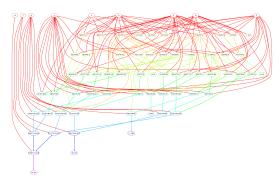
These DAGs often have MAXLIVE orders of magnitude larger than the number of registers available. We have solved this problem by developing a genetic algorithm (SUN-GA) that can restructure the code to drastically reduce MAXLIVE at the expense of performing a modest amount of redundant computation, with the amazing results summarized below:
