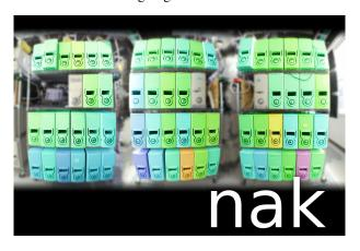
That's an actual photo of one of our clusters, NAK, tinted by **nodescape** as a real-time status display. Nodes are tinted from blue-to-green-to-red based on attribute values. As data ages (i.e., no new sensor readings are recorded), the tint increasingly dithers with magenta. A node with no data is tinted solid magenta.
